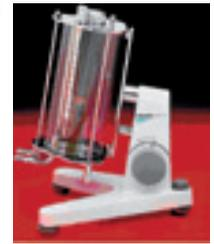
Absolute falling ball viscometer
